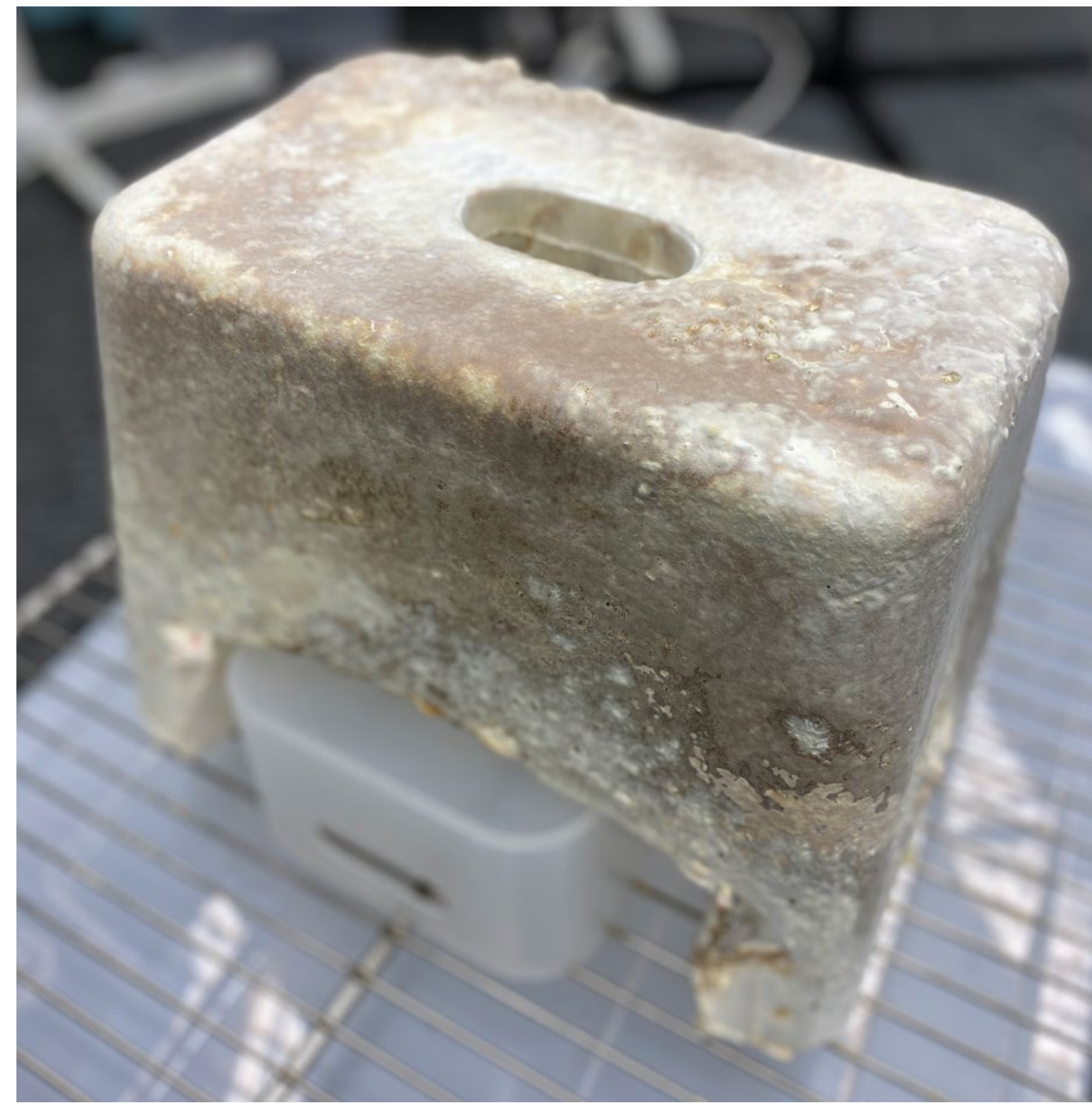
Figure 04. Mycelium composite stool right after it is baked in the oven. Photograph: Gyungju Chyon, 2023.
