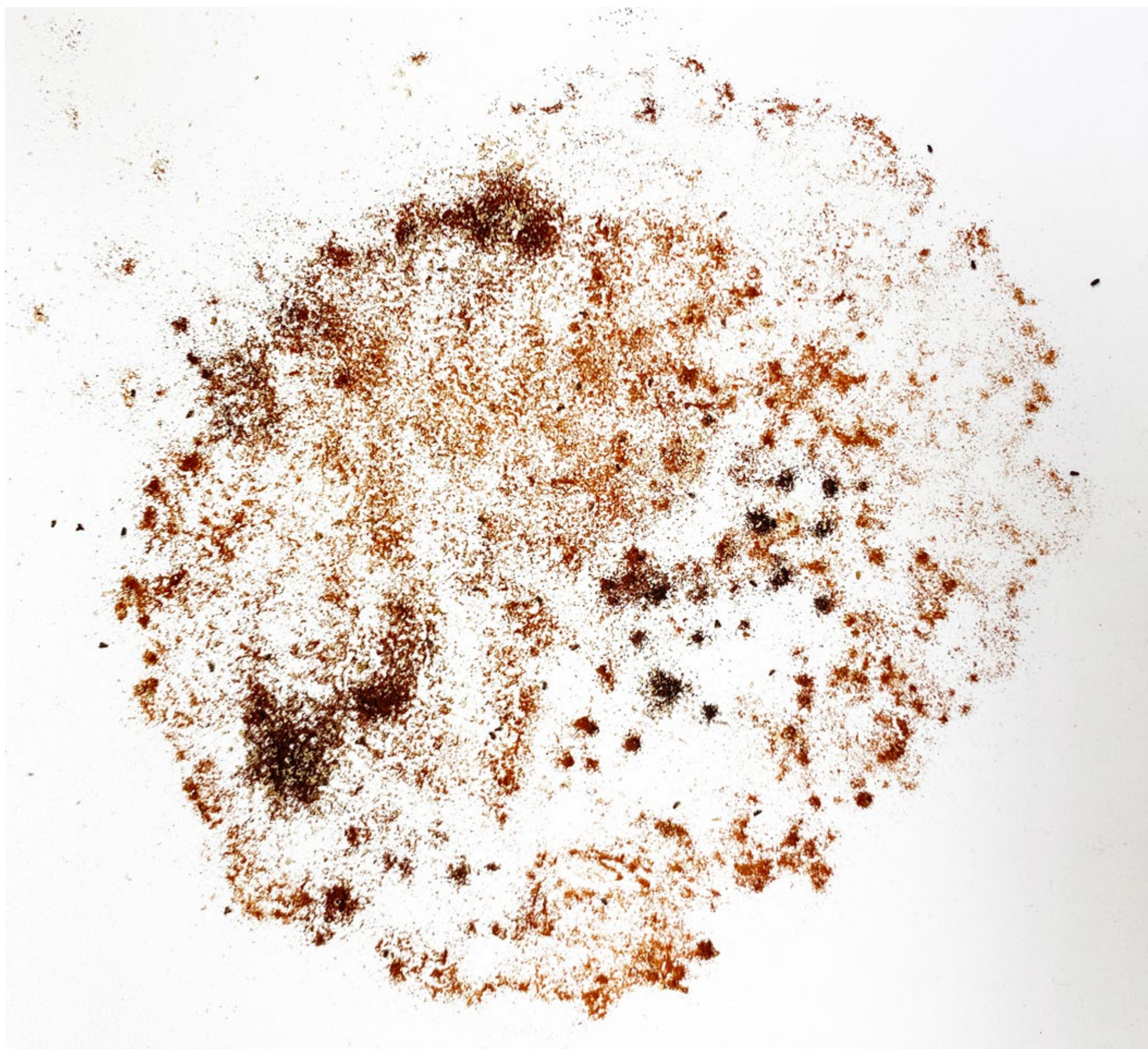
Figure 08. Fine wood dust from the sawdust, which makes up the mycelium composite, was found underneath the artefact. Photograph: Gyungju Chyon, 2024.
